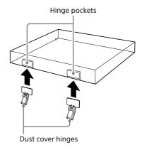
**2** Align the attached hinges with the hinge pockets on the rear of your turntable and push in the dust cover.
