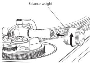
If a horizontal balance cannot be obtained because the cartridge is ٠ too heavy, attach the sub weight to the rear shaft of the tone arm.
