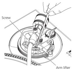
\* Turn the screw while pushing down this part.
