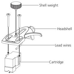
If a horizontal balance cannot be obtained because the cartridge is too light, use the supplied shell weight.
