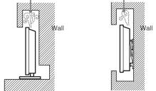
Inadequate ventilation can lead to overheating of the TV and may cause damage to your TV or cause a fire.
