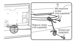
The length of the M4 machine screw differs depending on the rope or chain diameter. Please see below illustration.
