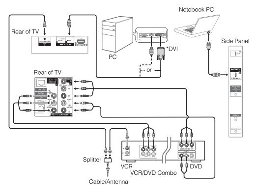
\* DVI does not support audio signals. Connect the audio output of the PC to the PC speakers or an A/V receiver to listen to sound from the PC.
