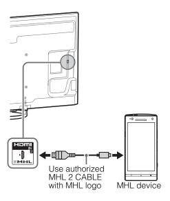
The MHL (Mobile High-Definition Link) enables the TV to communicate with a connected MHL-compatible device. The TV can charge the connected MHL-compatible device while playing photo/music/video from it. You can use the TV remote control to control the connected MHL-compatible device.
