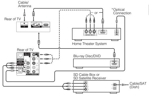
\* The optical connection is only needed for home theater system that do not support ARC (Audio Return Channel) when connecting with HDMI.
