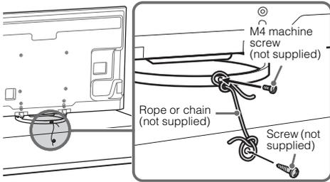
The length of the M4 machine screw differs depending on the rope or chain diameter. Please see below illustration.
