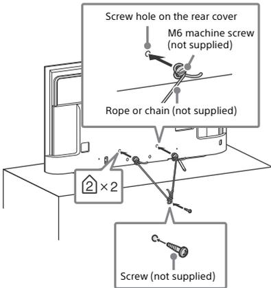
The length of the M6 machine screw differs depending on the rope or chain diameter. Please see below illustration.
