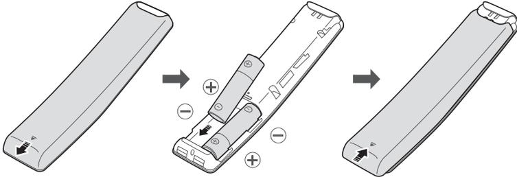
To install the batteries, push the rear cover open in the direction of the arrow, and then insert the batteries as shown in the figure. Make sure that the positive and negative ends are facing in the correct direction.
