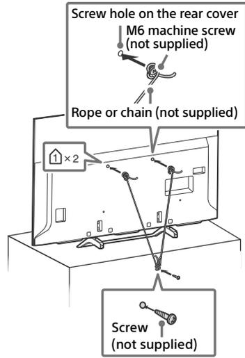
The length of the M6 machine screw differs depending on the rope or chain diameter. Please refer to below illustration.
