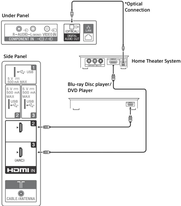
\* The optical connection is only needed for home theater system that do not support ARC (Audio Return Channel) when connecting with HDMI.
