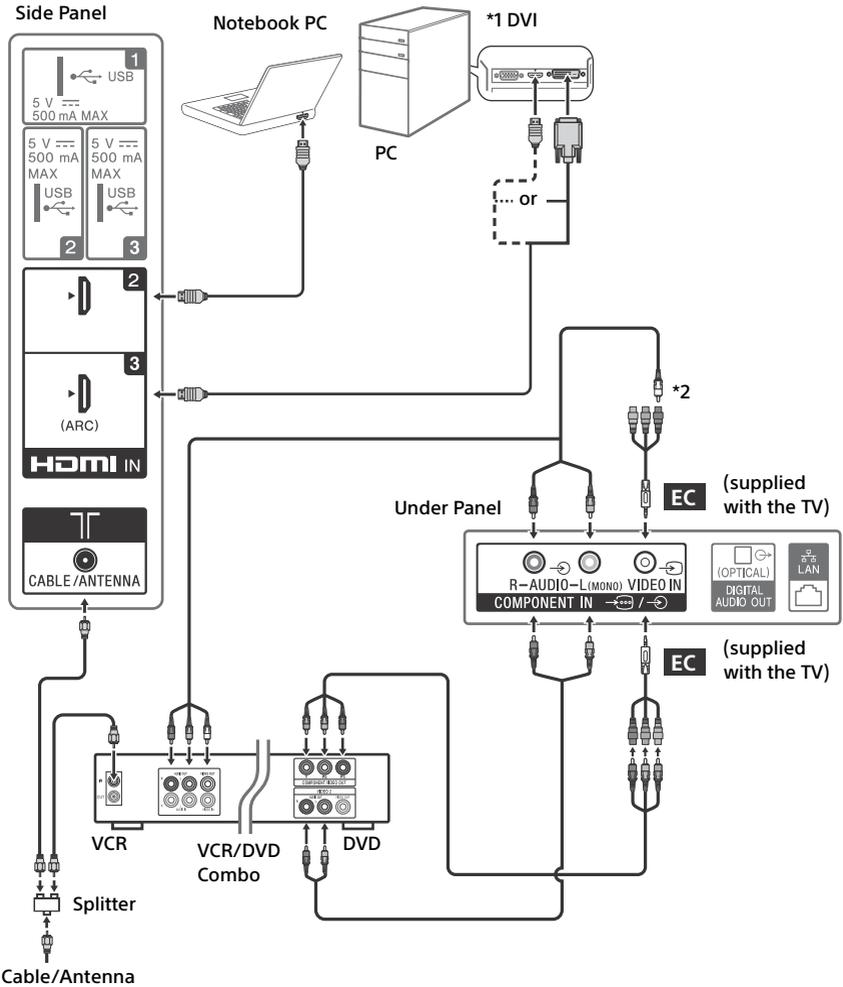
\*1 DVI does not support audio signals. Connect the audio output of the PC to the PC speakers or an A/V receiver to listen to sound from the PC.
