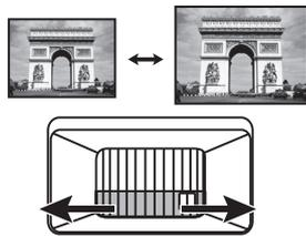
Sharpen the image by rotating the focus ring.
