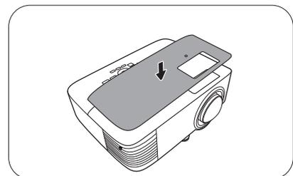
13. Tighten the screw that secures the lamp cover.
