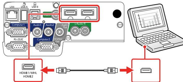
**Note:** The projector converts the digital audio signal sent from your computer into a mono analog signal for the internal speaker or a stereo analog signal if you are connecting to external speakers.
