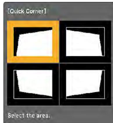
6. Use the arrow buttons on the projector or the remote control to select the corner of the image you want to adjust. Then press **Enter**.
