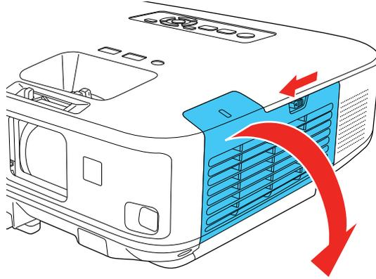
2. Pull the air filter out of the projector.
