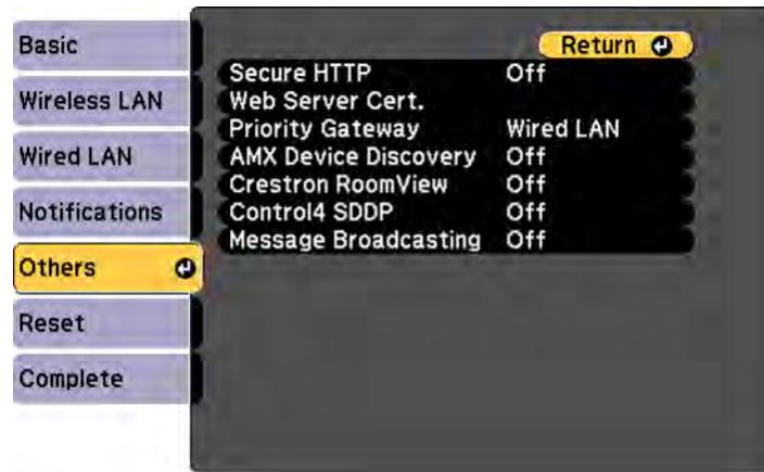
8. If you want to use the Secure HTTP protocol to encrypt communication when using Web Control, turn on the **Secure HTTP** setting and import the web server certificate using the **Web Server Cert.** setting.
