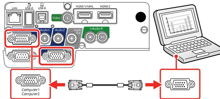
4. Tighten the screws on the VGA connector.
