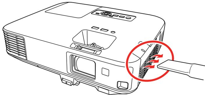
**Note:** You can remove the air filter so you can clean both sides of it. Do not rinse the air filter in water, or use any detergent or solvent to clean it.
