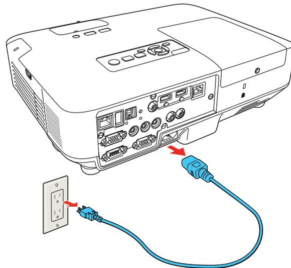
**Caution:** To avoid damaging the projector or lamp, never unplug the power cord when the Status light is on or flashing.
