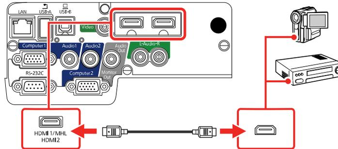
**Note:** The projector converts the digital audio signal sent from your video source into a mono analog signal for the internal speaker or a stereo analog signal if you are connecting to external speakers.
