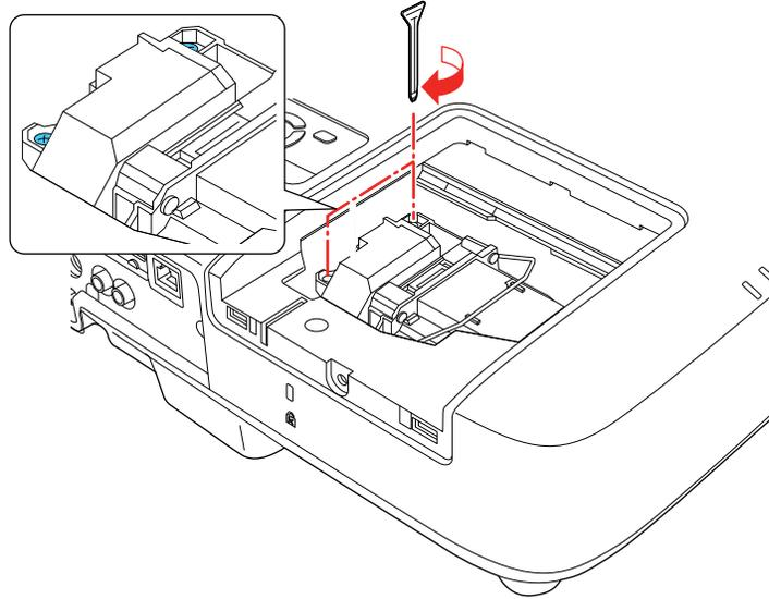
9. Replace the lamp cover and tighten the screw to secure it.
