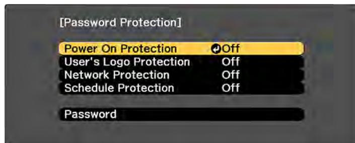
If you do not see this menu, hold down the **Freeze** button on the remote control for about seconds or until the menu appears.
