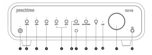
**On/Standby Button:** With the AC power cord connected and the rear panel **POWER** switch set to **ON**, this button toggles the unit between On mode (which selects the last input used) and Standby mode which lights the LED red.
