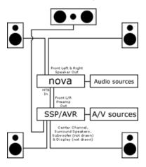
Connect Line-level (RCA style) front left and right outputs from the SSP or AVR to the **AUX-1/HTB** input on the nova.
