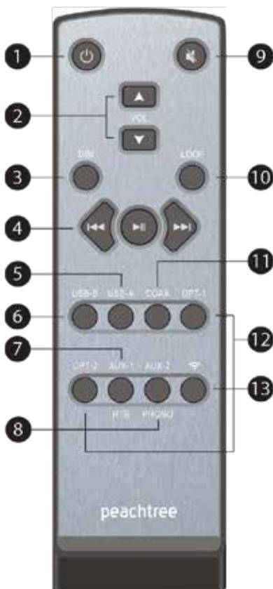
❶ **On/Standby Button:** With the AC power cord connected and the rear panel **POWER** switch set to **ON**, this button toggles the unit between On mode (which selects the last input used) and Standby mode which lights the LED red. *Note: it takes ~2 seconds for the unit to fully transition from standby to on mode. During this time, any commands will not be acknowledged.*
