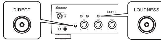
When this condition is set to ON, the **STANDBY/APD** indicator on the unit's front panel will light green. Press the buttons again to disable the setting.
