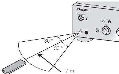
Keep in mind the following when using the remote control:
