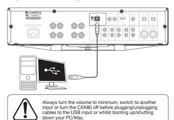
Note: Always use a high quality USB connection cable certified as USB Hi- Speed. USB cable connections longer than 3m may result in inconsistent audio performance.
