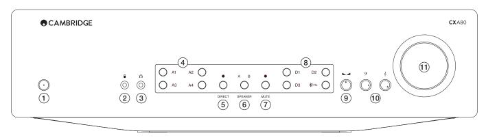
Note: Selected sources and functions are represented by a Blue light. MP3 jack input is represented by an Orange 'A4' light. CXA80 has additional Orange lights for USB and Balanced inputs.
