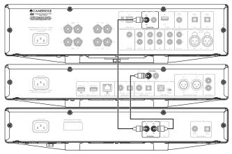
Adding an additional connection from CXN to CXA will enable the use of the Cambridge Connect app function.
