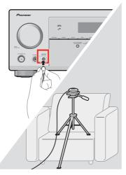
If you have a tripod, use it to place the microphone so that it's about ear level at your normal listening position. Otherwise, place the microphone at ear level using a table or a chair. Press BD button on the remote control to switch to BD/ DVD entry.
