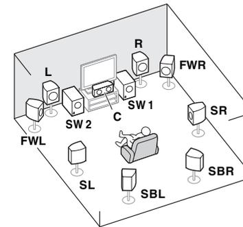
This plan replaces the left and right front height speakers shown in [A] with the left and right front wide speakers (**FWL/FWR**).
