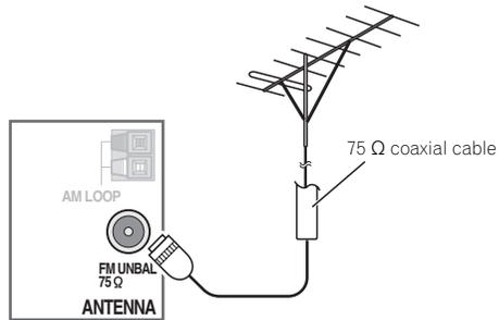
To improve AM reception, connect a 5 m to 6 m (16 ft. to 20 ft.) length of vinyl-coated wire to the **AM LOOP** terminals without disconnecting the supplied AM loop antenna. For the best possible reception, suspend horizontally outdoors.
