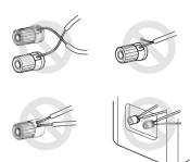
When using commercially available banana plugs: tighten the speaker terminals to the end and then insert the banana plugs. Do not insert the core of speaker cable directly into the hole for banana plug of speaker terminal. (North American model)
