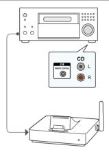
Connect an Onkyo component with RI jack to this unit using an RI cable and an analog audio cable. For details, refer to the instruction manual of the component with RI jack. The RI cable can be connected in any order. When there are two RI jacks, both jacks work in the same way and are interchangeable.
