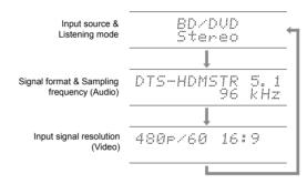
If "Dolby D 5.1" is displayed in Signal format, the Dolby Digital 5.1 ch signals are being input. When listening to AM/FM radio, the band, frequency and preset number are displayed.
