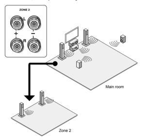
These settings are required: After connecting the speakers, press RCV and then SETUP on the remote controller, select "2. Speaker" - "Configuration" and set "Powered Zone 2" to "Yes".
