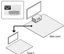
Settings are required: Press RCV and then Output Assign" - "TV Out" and set the "Zone 2 HDMI" setting to "Use".
