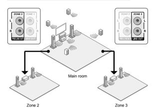
Zone 2 audio can be adjusted with both the unit and the pre-main amplifier used in the separate room. Zone 3 audio should be adjusted with the pre-main amplifier used in the separate room.
