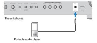
If you select "AUX" as the input source by pressing AUX, the audio played back on the device will be output from the unit.
