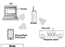
To use this function, the unit and your PC or iPhone must be connected to the same router (p. 13). You can check whether the network parameters (such as the IP address) are properly assigned to the unit in "Information" (p. 40) in the "SETUP" menu.
