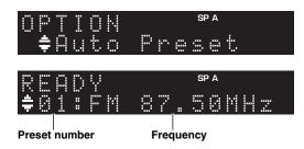
This unit starts scanning the FM band about 5 seconds later from the lowest frequency upwards. To begin scanning immediately, press ENTER.
