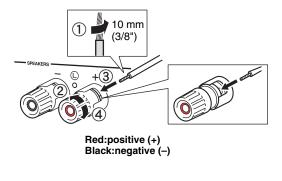
When inserting speaker cables into the speaker terminals, insert only the bare speaker wire. If insulated cable is inserted, the connection may be poor and sound may not be heard.  Connecting via banana plug (North America, Australia, General models only)
