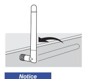
Do not apply excessive force on the wireless antenna. Doing so may damage the antenna.
