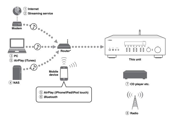
\* You need a commercially available wireless router (access point) when you use a mobile device.
