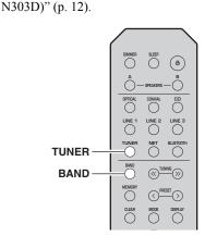
1 Press TUNER to select "TUNER" as the input source.
