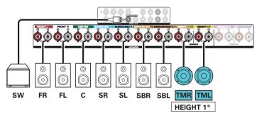
\* The top front or top rear speakers can be connected instead of the top middle speakers. In this case, set the ceiling speakers to be connected under "Height" - "Layout" in the menu. (\*\*\* p. 225)
