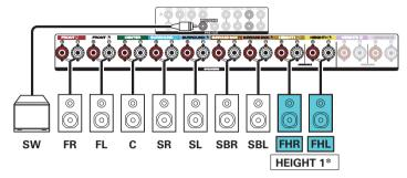
\* The rear height speakers can be connected instead of the front height speakers. In this case, set the height speakers to be connected under "Height" - "Layout" in the menu. (1287 p. 225)
