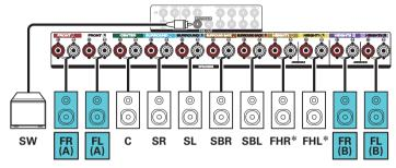
\* The height speakers, ceiling speakers and Dolby Atmos Enabled speakers can be connected to the HEIGHT1 speaker terminals. Set the speaker to be connected from "Height" - "Layout" in the menu. (125 p. 225)
