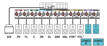
\* The height speakers, ceiling speakers and Dolby Atmos Enabled speakers can be connected to the HEIGHT1 speaker terminals. Set the speaker to be connected from "Height" - "Layout" in the menu. ( ) 225)
