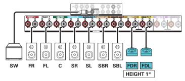
\* The surround Dolby or back Dolby speakers can be connected instead of the front Dolby speakers. In this case, set the Dolby Atmos Enabled speakers to be connected under "Height" - "Layout" in the menu. (12) p. 225)
