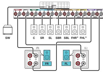
\* The height speakers, ceiling speakers and Dolby Atmos Enabled speakers can be connected to the HEIGHT1 speaker terminals. Set the speaker to be connected from "Height" - "Layout" in the menu. ( Layout ) 225)
