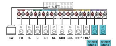
\* The height speakers, ceiling speakers and Dolby Atmos Enabled speakers can be connected to the HEIGHT1 speaker terminals. Set the speaker to be connected from "Height" - "Layout" in the menu. (127 p. 225)
