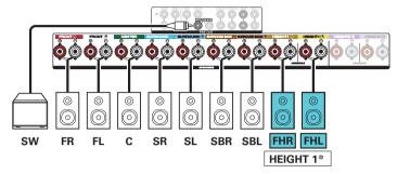
\* The rear height speakers can be connected instead of the front height speakers. In this case, set the height speakers to be connected under "Height" - "Layout" in the menu. (1287 p. 220)
