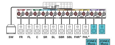
\* The height speakers, ceiling speakers and Dolby Atmos Enabled speakers can be connected to the HEIGHT1 speaker terminals. Set the speaker to be connected from "Height" - "Layout" in the menu. (127 p. 220)
