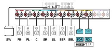
\* The surround Dolby speakers can be connected instead of the front Dolby speakers. In this case, set the Dolby Atmos Enabled speakers to be connected under "Height" - "Layout" in the menu. ( \*\* p. 220)
