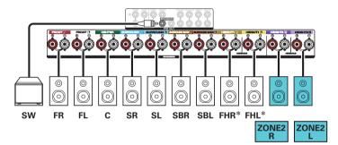
\* The height speakers, ceiling speakers and Dolby Atmos Enabled speakers can be connected to the HEIGHT1 speaker terminals. Set the speaker to be connected from "Height" - "Layout" in the menu. ( ) 220)
