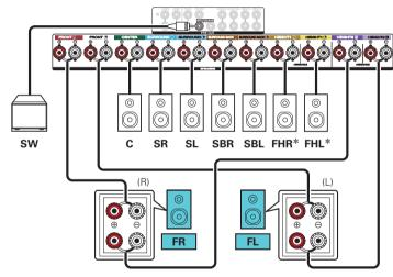
\* The height speakers, ceiling speakers and Dolby Atmos Enabled speakers can be connected to the HEIGHT1 speaker terminals. Set the speaker to be connected from "Height" - "Layout" in the menu. ( ) 220)
