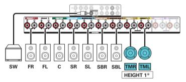
\* The top front or top rear speakers can be connected instead of the top middle speakers. In this case, set the ceiling speakers to be connected under "Height" - "Layout" in the menu. ( \*\*P p. 220)
