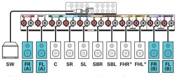
\* The height speakers, ceiling speakers and Dolby Atmos Enabled speakers can be connected to the HEIGHT1 speaker terminals. Set the speaker to be connected from "Height" - "Layout" in the menu. (127 p. 220)
