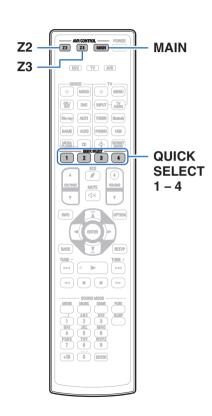
Settings such as the input source, volume level and sound mode can be registered to the QUICK SELECT 1 - 4 buttons.
