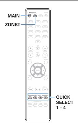
Settings such as the input source, volume level and sound mode can be registered to the QUICK SELECT 1 - 4 buttons.
